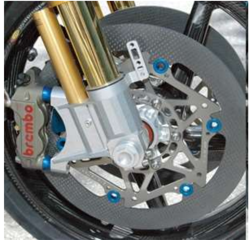
Ceramic Matrix Composite (CMC) rotor
